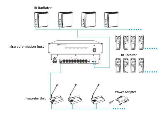
1. Install the host in a standard rack, the radiation panel is installed in the corner of the room, as far as possible to keep radiation to the every corner.
