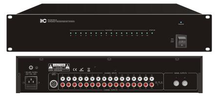
TS-0670H series digital infrared emission host is the core part of the digital infrared voice distribution system. With fully digital DQPSK modulated transmission and digital audio compression coding system, it can transmit the 8 channels languages at the same time. Infrared emission host can be installed on the 19-inch standard rack, easy to storage and preservation.
