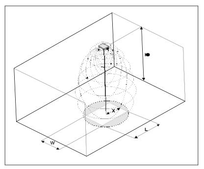
Picture 4-8-2 Typical rectangular floor area by 90 degree
