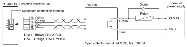
Note: Cut out the control cables if they are not used to avoid short-circuiting.
