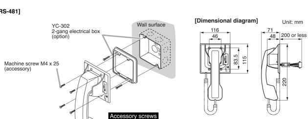
The RS-480/481 come with 2 types of screws to match the box screw threads: M4 x 25 and UNC No. 6-32 x 18.
