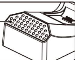
The LED Charge Indicator on the Charging Station displays the charging status.
