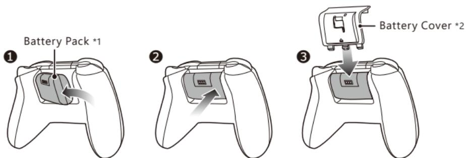
\*1 Properly insert the battery pack aligned correctly.
