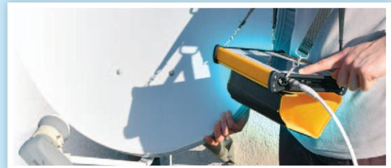
The **HD RANGER *UltraLite*** is a universal field strength meter that covers a comprehensive mix of broadcast standards around the globe.
